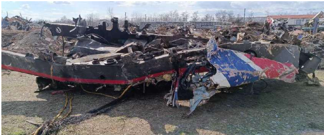
Figure 17. Part (chassis) of the completely destroyed locomotive 120-023 of the passenger train IC-62.
