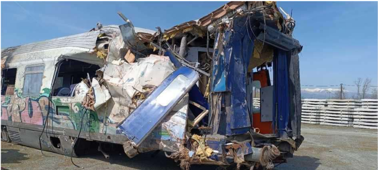
Figure 88. Position 5) B3 2nd class coach, derailed and went down a slope, lost bogies, no other damage from derailment or crash, specific impact damage from B2 coming down from above.
