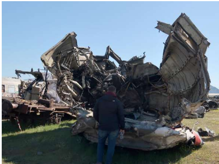
Figure 16. Front view of the locomotive 120-022, roof missing.
